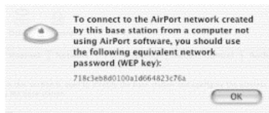
Figure B-13. Printing out the WEP key in hexadecimal for use by non-Apple 802.11 stations
